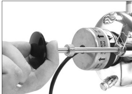
Step 2 – Gently pull wiper knob out
